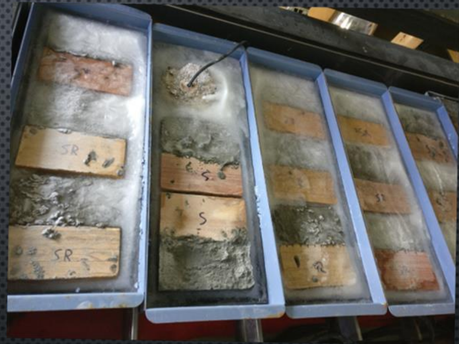
Figure 4: Freeze-thaw machine at coldest point in cycle [6]
