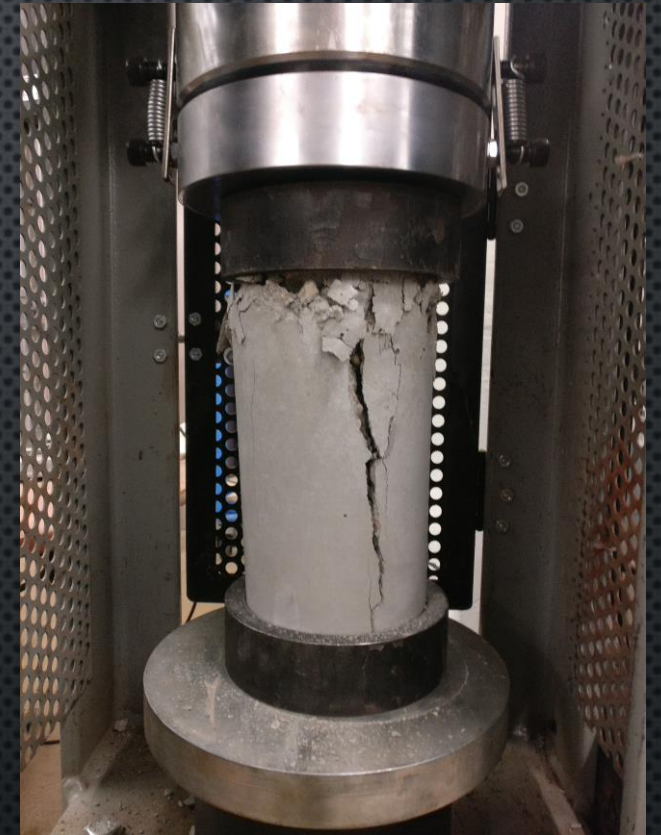
Figure 10: 7 day cure compression failure [14]
