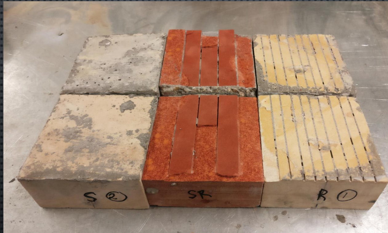
Figure 18: The failed interfaces of the smooth, semi-rough, and rough specimen interfaces [20]
