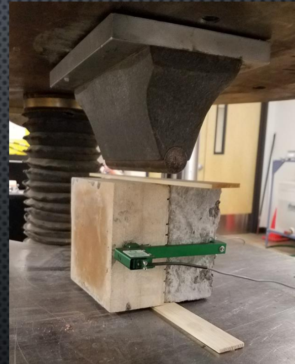
Figure 15: Specimen, before test, with placed extensometers on each side [17]
