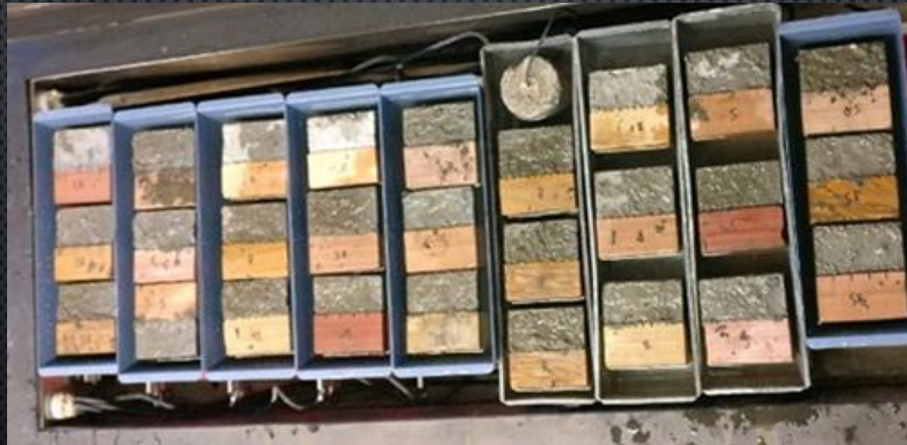
Figures 11: Specimens undergoing freeze - thaw cycles [15]
