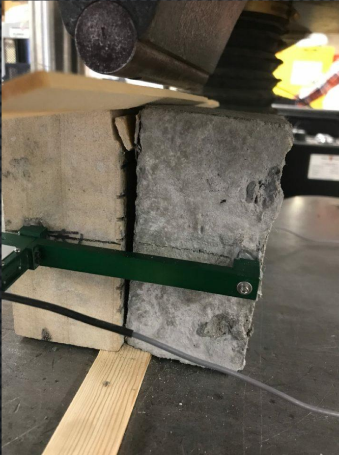
Figure 16: Specimen tensile failure [18]
