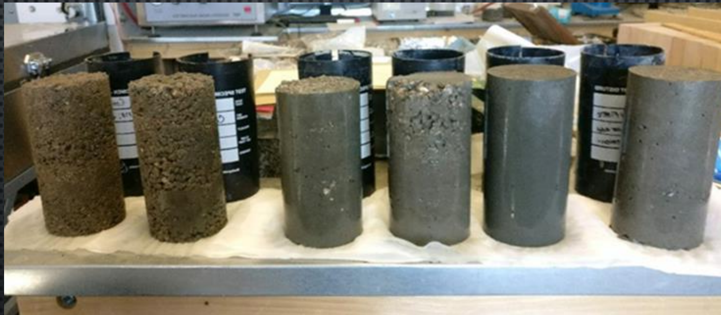
Figure 7: Specimens for preliminary testing, original design mix (farthest left), modification improvements (left to right) [9]
